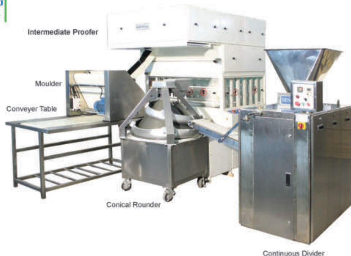
LINE 1) Capacity:1800pcs/Hr;Dough Weight Range:100-300g
