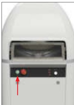
4. Close the guard casing. Press the green Start key
