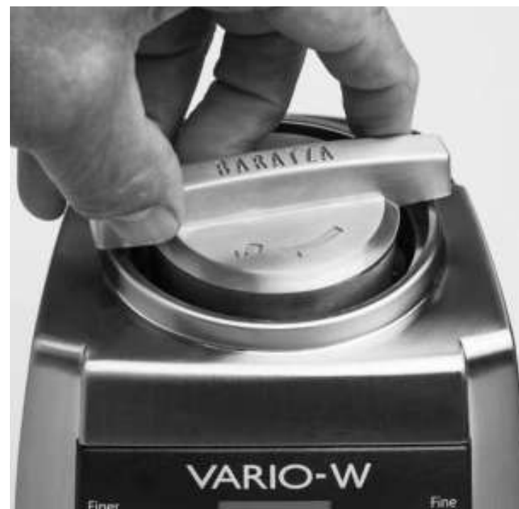
Rotate Baratza burr tool clockwise to remove the burr carrier.
