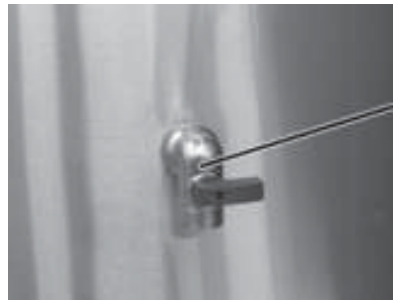
1. Control valve of steam jacket
