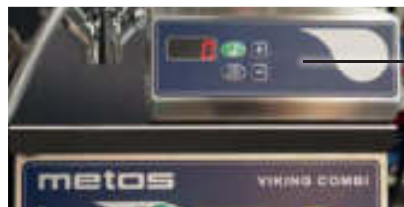
Automatic water filling unit
