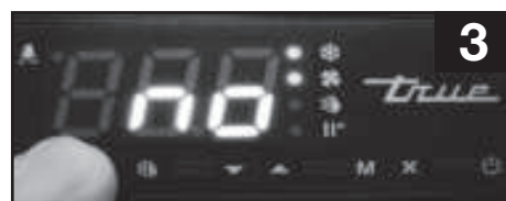
Image 3: If "no" appears on screen, the controller is unlocked.
