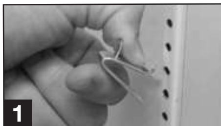
(Installing top tab of shelf clip)
