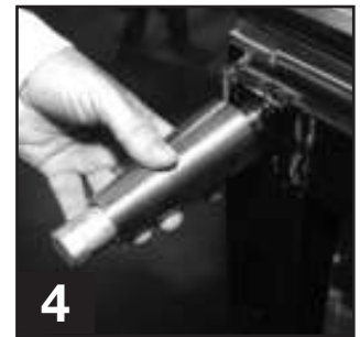
4 Thread leg into cabinet bottom frame rail.
