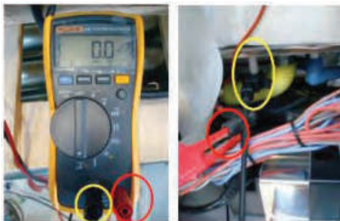
Figure 21 Multimeter connection to the flame control plug
